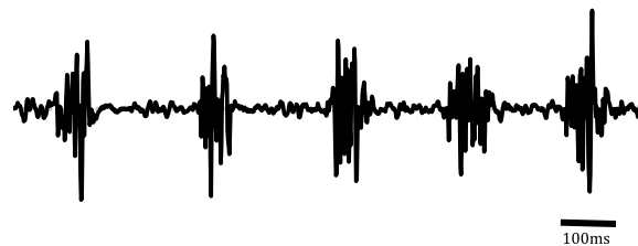
Figure 5.1: An example of the EMG bursts. Here we have 5 EMG bursts in this example. Each EMG burst is repetitive muscle contractions and between two EMG bursts there is a silent region.
